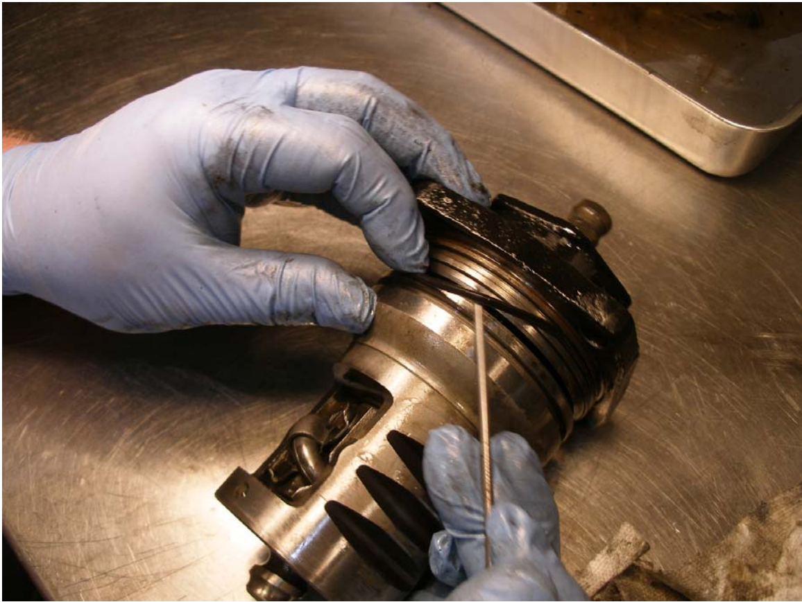
13. Install new O rings and finally the Teflon seal.
