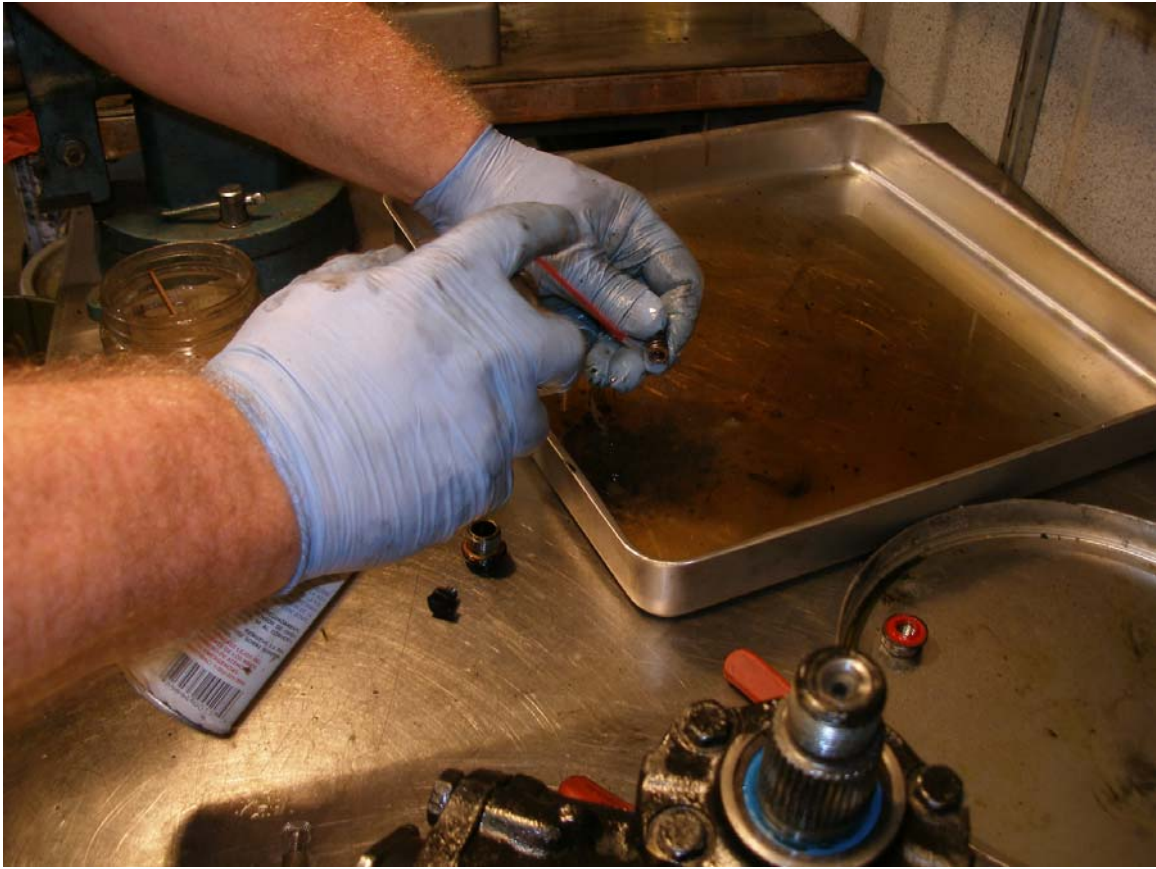
52. Replace copper seal washer.
