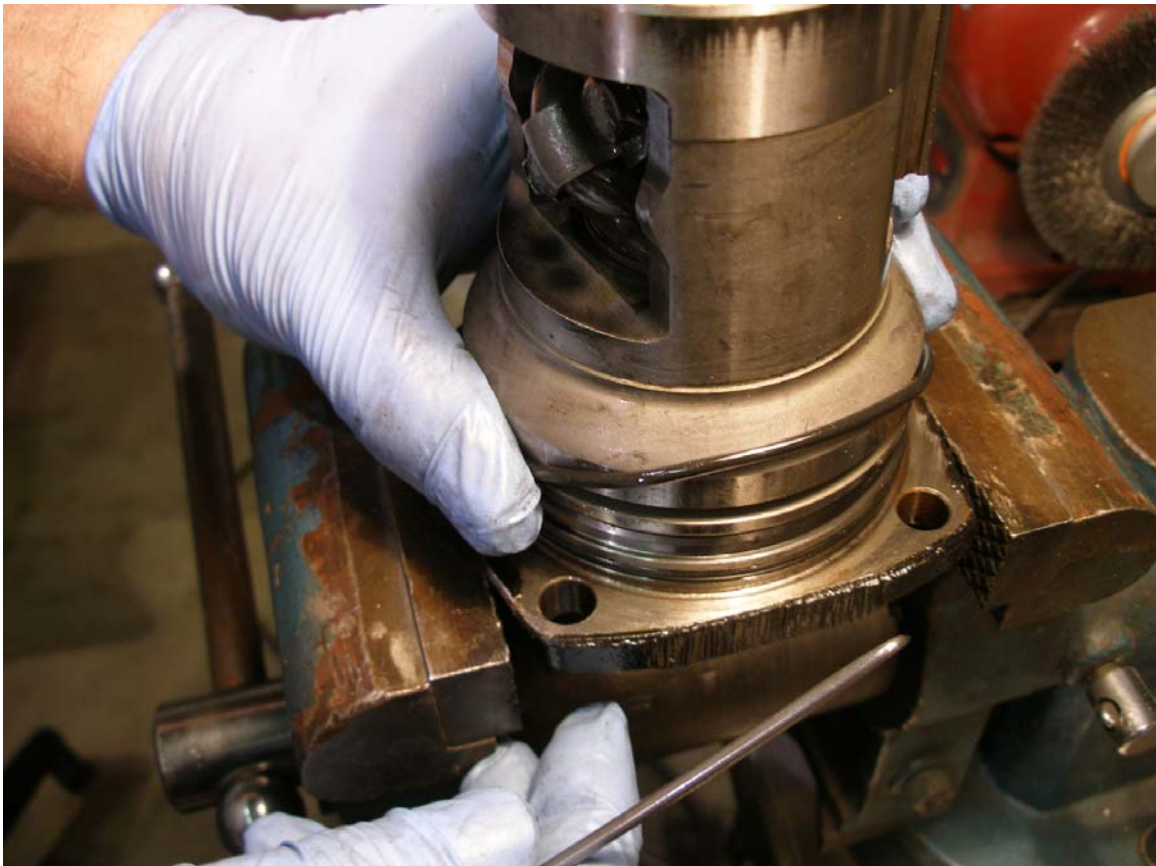
13. Install new O rings and finally the Teflon seal.
