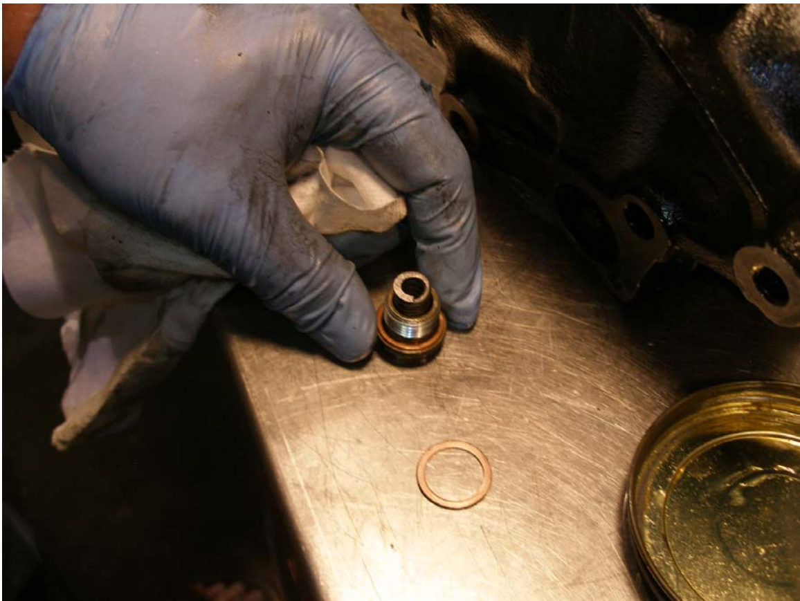
52. Replace copper seal washer.
